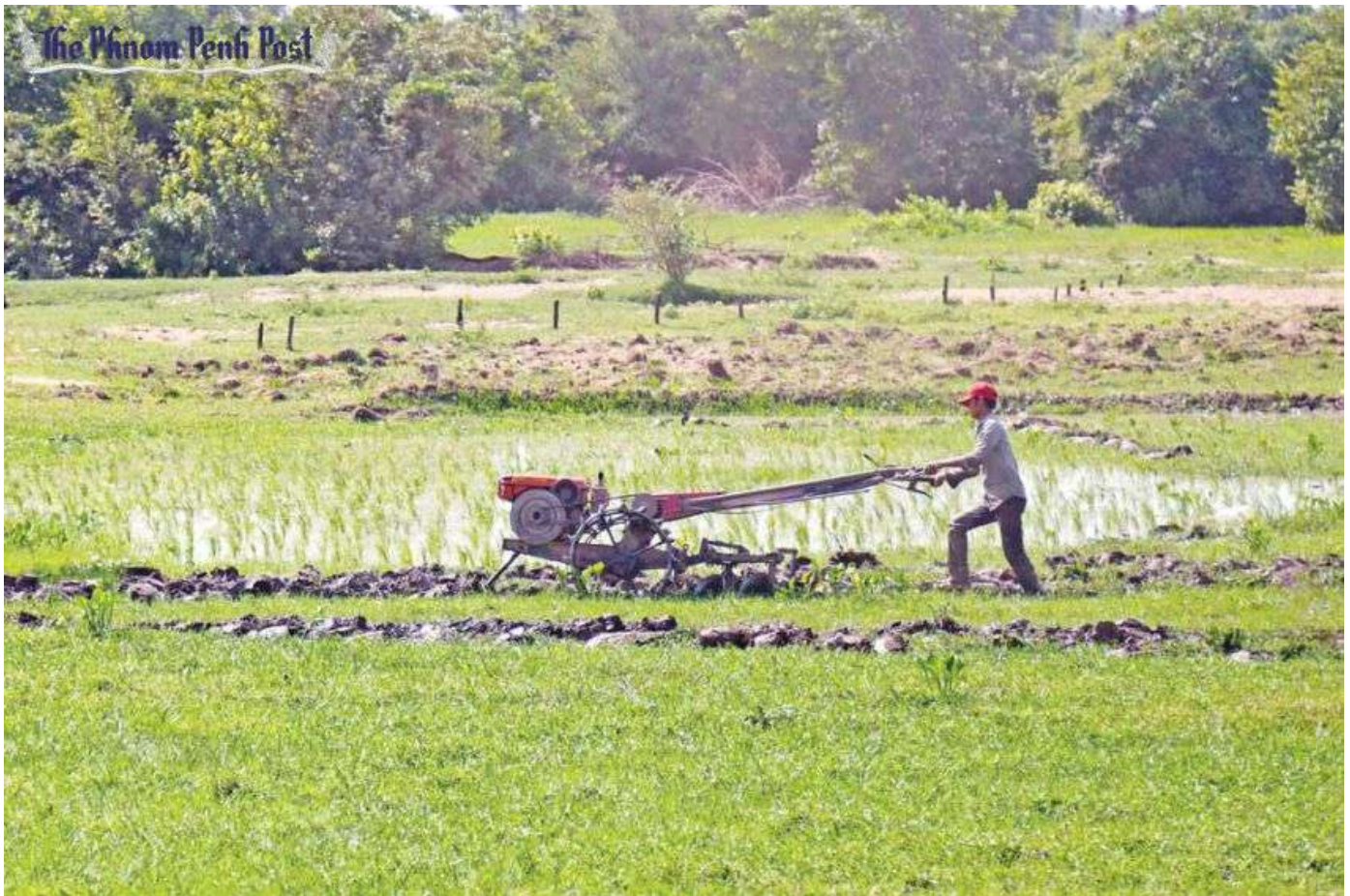
A man uses a single-axle hand tractor to plough his field in Kampong Speu province last year. Hong Menea
